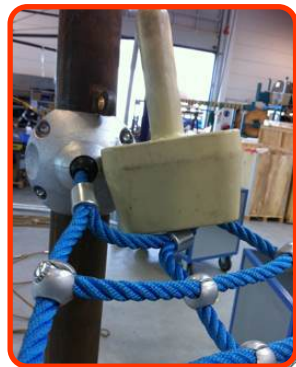
Rope Platform trap test
